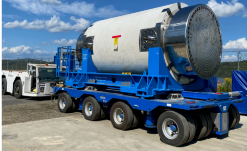
Moving loaded Transfer Trailer with the "Tugger"
